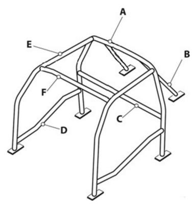
A Six Point Rollcage must have the following components as a minimum and in the positions illustrated in the image above.
